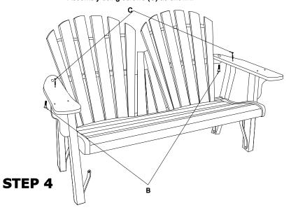
Attach Arms to Back Legs from the top using screws (C). Bolt Arm Assemblies to Back Assembly using Bolts (B) as shown. Then, tighten the leg bolts.
