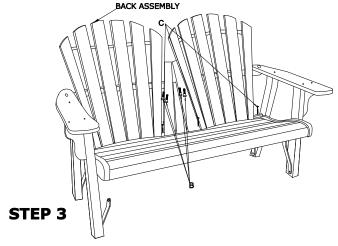
From behind, attach Center Back Assembly to the other Back Assembly using chair bolts (B), then attach Back Assembly to Seat Assembly using screws (C) as shown.
