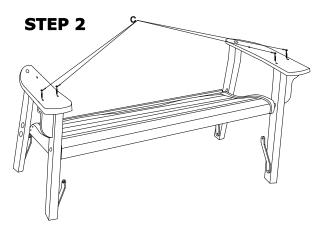
Attach Arms to Front Legs using screws (C) as shown.
