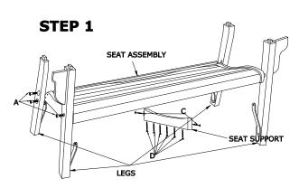
Attach Seat Support to Seat Assembly from the bottom using screws (D), and from the front and back using screws (C), as shown. Attach Side Assemblies to Seat Assembly using bolts (A) as shown. Only hand tighten the bolts.
