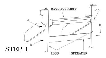
Attach spreader to legs with screws (B) as shown. Bolt legs to base assembly using bolts (A).
