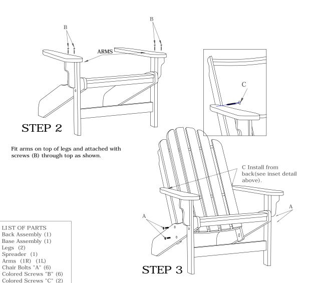
Bolt back assembly to base assembly using 2 bolts (A) on each side as shown. Attach arm to seat back using Large Head Screws (C).
