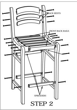
Step 2. Place spreaders into mortise (pocket) inside assemblies as shown. Loosely attach with screws "A." Follow this procedure with rails and slats, followed by back rests.
