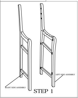
Step 1. Align right and left side assemblies as shown.
