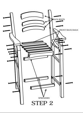
Step 2. Place spreaders into mortise (pocket) inside assemblies as shown. Loosely attach with screws "A." Follow this procedure with rails and slats, followed by back rests.
