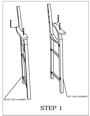
Step 1. Align right and left side assemblies as shown, and attach arms.
