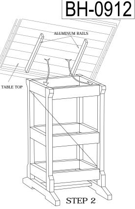
Place the table top on the base so that the Aluminum Rails on the table top fit with in the base as shown above
