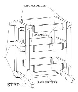
Attach Side Assemblies to Spreaders by placing the tenon into the mortise (pocket) and attching with screws (A) as shown.
