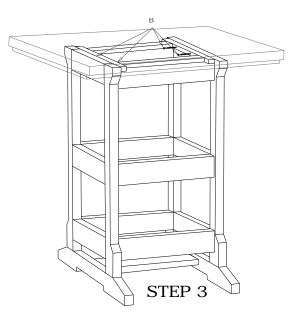
Attach Table Top to base using uncolored screws (B). From the underside screw through pre-drilled holes in the aluminum rails into base assembly.
