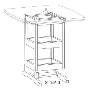
Attach Table Top to base using uncolored screws (B). From the underside screw through pre-drilled holes in the aluminum rails into base assembly.
