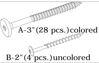
LIST OF PARTS Side Assemblies (2) Spreaders (6) Base Spreader (1) Table Top (1) Colored Screws "A" (28) Un-Colored Screws "B" (4) Insert Bit Tool (1)
