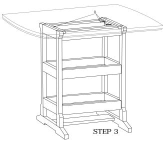
Attach Table Top to base using uncolored screws (B). From the underside screw through pre-drilled holes in the aluminum rails into base assembly.
