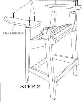
Attach arm rest and supports as shown.
