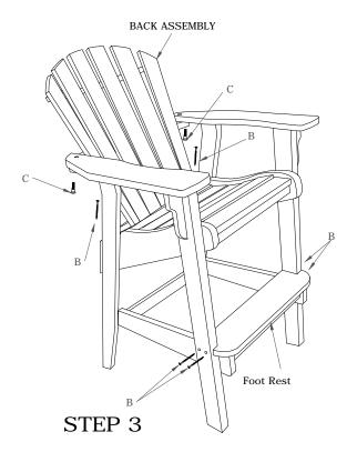
Slide back onto seat and attach at seat and arm rest. Attach foot rest.
