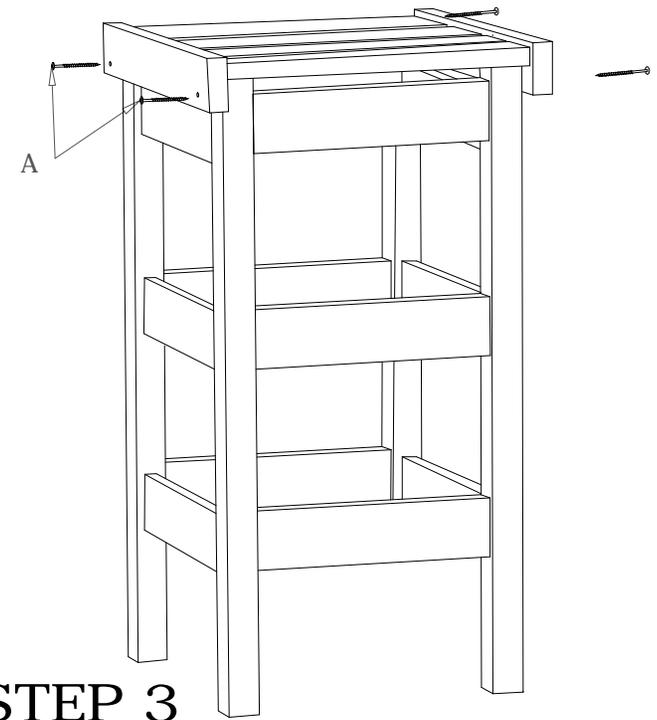
Attach Side Assemblies to Spreaders by placing the tenon into the mortise (pocket) and attaching with screws (A) as shown.
