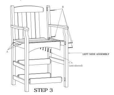
Fit seat slats into chair as shown. From the bottom side use uncolored screws (C) to secure slats. Use screws (A) to attach Side Assemblies to Slats.
