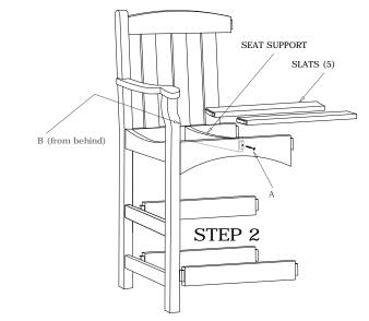
Attach Seat Supports using a screw (A) in the front and screw (B) in the back. Install Slats into slots provided on Right Side Assembly.
