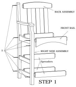
Attach Back Assembly and Front Rail to Right Side Assembly using screws (B) as shown.
