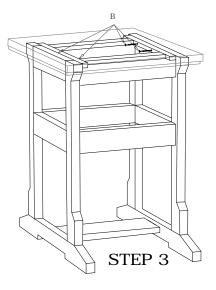
Attach Table Top to base using uncolored screws (B). From the underside screw through pre-drilled holes in the aluminum rails into base assembly.
