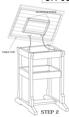
Place the table top on the base so that the Aluminum Rails on the table top fit with in the base as shown above
