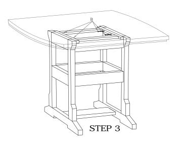
Attach Table Top to base using uncolored screws (B). From the underside screw through pre-drilled holes in the aluminum frame into base assembly.
