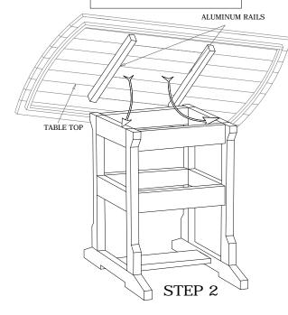
Attach Side Assemblies to Spreaders by placing the tenon into the mortise (pocket) and attching with screws (A) as shown.
