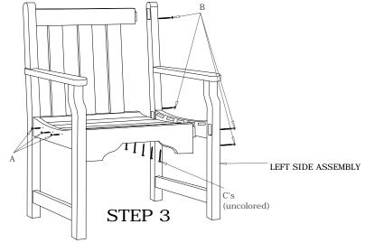
Fit seat slats into chair as shown. From the bottom side use uncolored screws (C) to secure slats. Use screws (A) to attach Side Assemblies to Slats.
