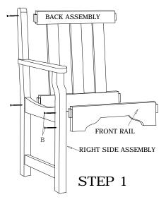
Attach Back Assemblies and Front Rail to Right Side Assembly using screws (B) as shown.
