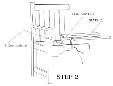
Attach Seat Supports using a screw (A) in the front and screw (B) in the back. Install Slats into slots provided on Right Side Assembly.
