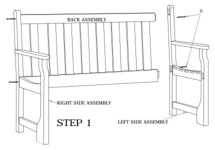
Attach Side Assemblies to Back Assemblies using screws (B) as shown.
