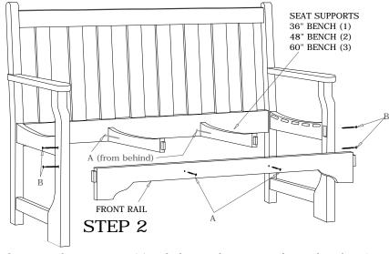
Attach Front Rail using screws (B) with the metal support to the inside. Place Seat Supports in place and screw through Back Assembly with screws (B) and through front rail with screws (A).
