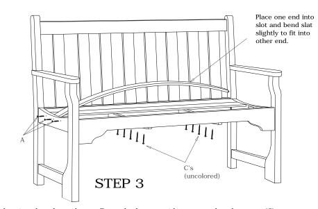
Fit seat slats into bench as shown. From the bottom side use uncolored screws (C) to secure slats. Use screws (A) to attach Side Assemblies to Slats.
