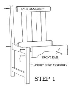
Attach Back Assemblies and Front Rail to Right Side Assembly using screws (B) as shown.
