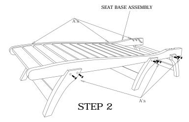
Arrange Front Leg Assemblies and Back Leg Assembly.
