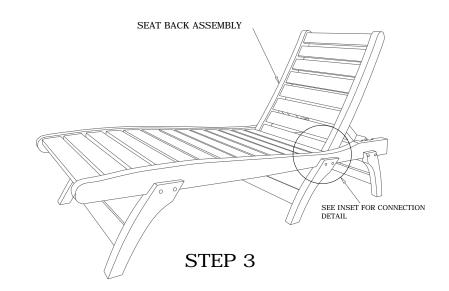
Attach Seat Back to Seat Base using Screws (B) and Nylon Washers (C). as shown in inset detail.
