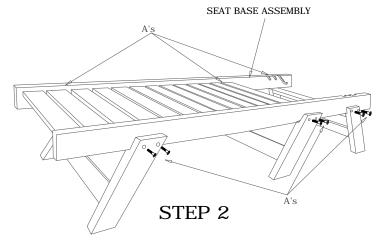
Attach Seat Base Assembly to legs using Chair Bolts (A)..
