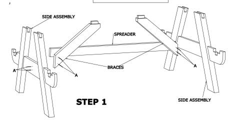
Attached Braces to Side Assemblies by placing tenon into pocket and attaching with screw (A) as shown. Attach Spreader to Braces using screws (A) as shown.
