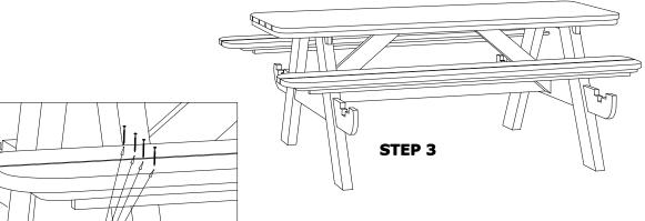
Place Seats onto side assemblies and attach with screws (A) as show.
