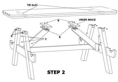
Fit the pocket in the Under Brace to the tenon on the Brace. Attach from the top with Screws (B) as shown. Place the table top on the Assembly. Insure the Tie Slats fit into the slots in the Side Assemblies and attach with Bolts (D) as Shown. Place Screws (C) into Side Assemblies as shown. From the underside using screws (B) screw trough holes in Under Brace into bottom of table.
