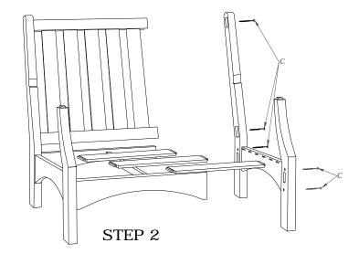
Using the detail in the drawing above, place the tenon on the center support into the slot on the front and back spreaders. Attach with screws "B". Lay the right side assembly on the floor with the pockets face up. Insert the Spreader into the pockets as shown. Insert the back assembly into the pockets as shown. Stand assembly up and attach with screws "C" as shown.
