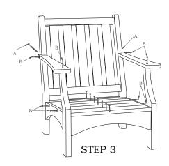
Attach slats on both sides and seat with screws "B". Place the Arm Rest as shown and attach the top and sides with screws "B" and through the back with screw "A"
