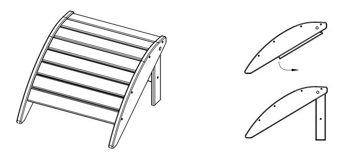
**1.** Remove Part A from the box and pivot the legs down as shown
