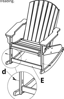
**7.** Turn the back/seat assembly on it's side. Lay one arm/leg assembly from steps 1-5 on the back/seat assembly and fasten using 1 each of hardware a & b as shown. Lay Part H in place and fasten with 2 of hardware b at the back, then 1 hardware b at the front. Flip the chair to the opposite side and repeat this process.
