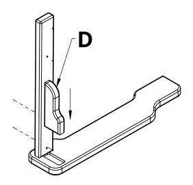
**4.** &Using hardware c, attach Part D as shown.
