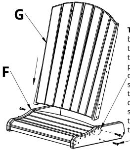
Tip: If the seat back is a little tight going into the seat base, partially loosen 2 of the seat screws to allow the base legs to open, insert the seat back and then re-tighten the screws.
