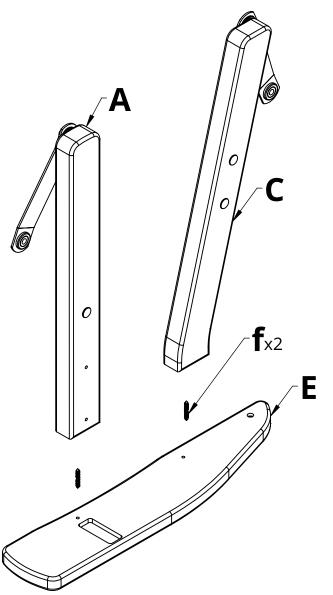
**1.** Starting with Part C, attach Parts C & A to Part E by inserting Hardware f into the predrilled holes and rotating clockwise, stopping when the assembly is tight
