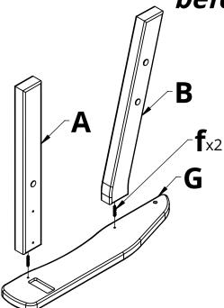
**1.** Attach PartS A & B to Part G by inserting Hardware f into the pre-drilled holes and rotating Parts A & B clockwise, stopping when the assembly is tight
