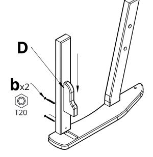
**2.** Attach Part D to the previous assemblies using Hardware b
