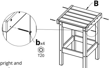
**4.** Stand the asssembly upright and connect Part B with Hardware b
