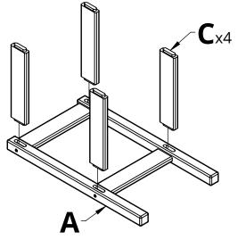
**1.** Place Part A on its side and insert Parts C into place as shown
