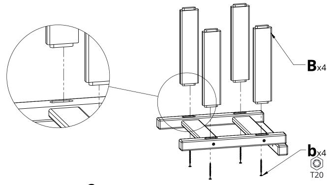
**2.** Place second Part A on assembled piece from Step 1,attach with Hardware b
