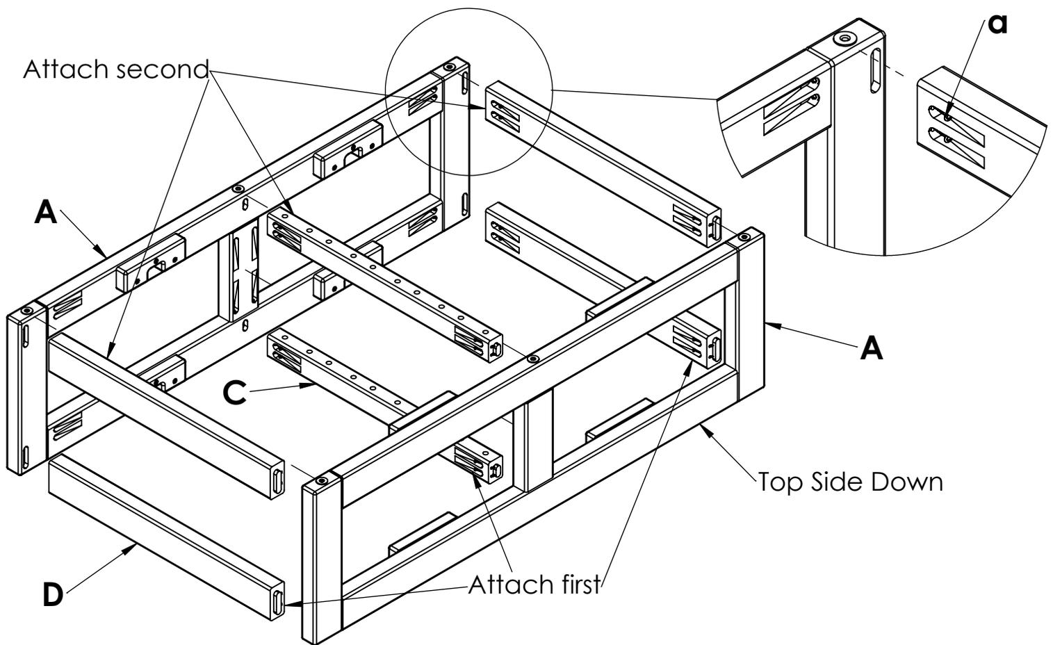
**1.** With the leg assemblies (**A**) upside-down on a flat surface, attach parts **C** & **D** in the orientation shown using hardware **a** and the bit provided. It will help to attach the **C** & **D** parts nearest the ground on one leg assembly, then attach the opposite leg. Then attach the remaining **C** & **D** away from the ground last.
