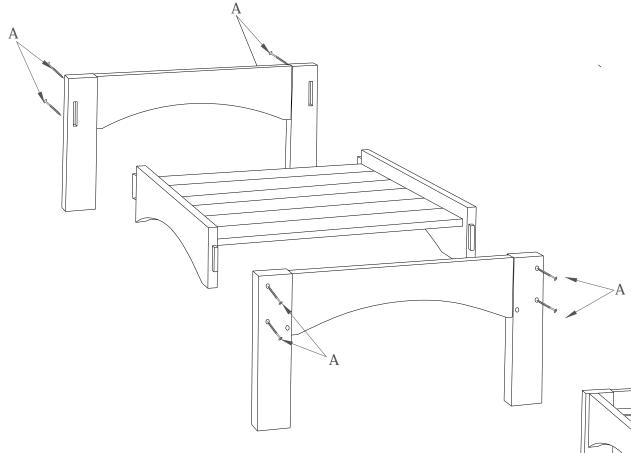
Place tenon in Shelf Assembly into Slots in Leg Assemblies. Attach with Screw "A" as shown above.
