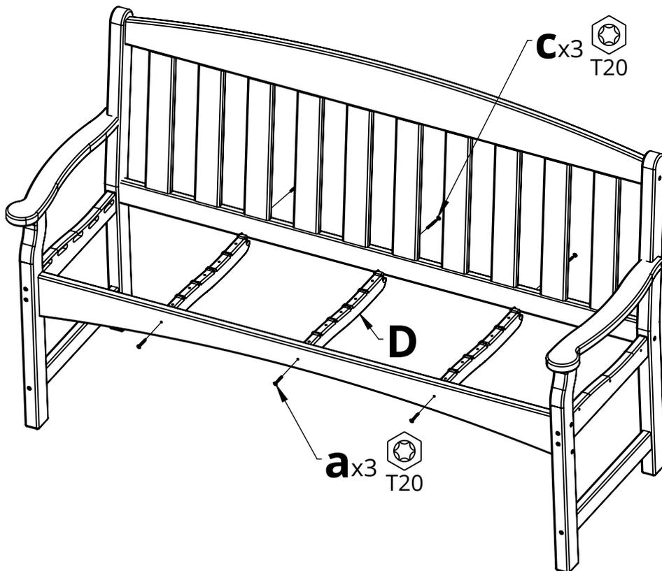
2. Connect Parts D to the previous assembly as shown
