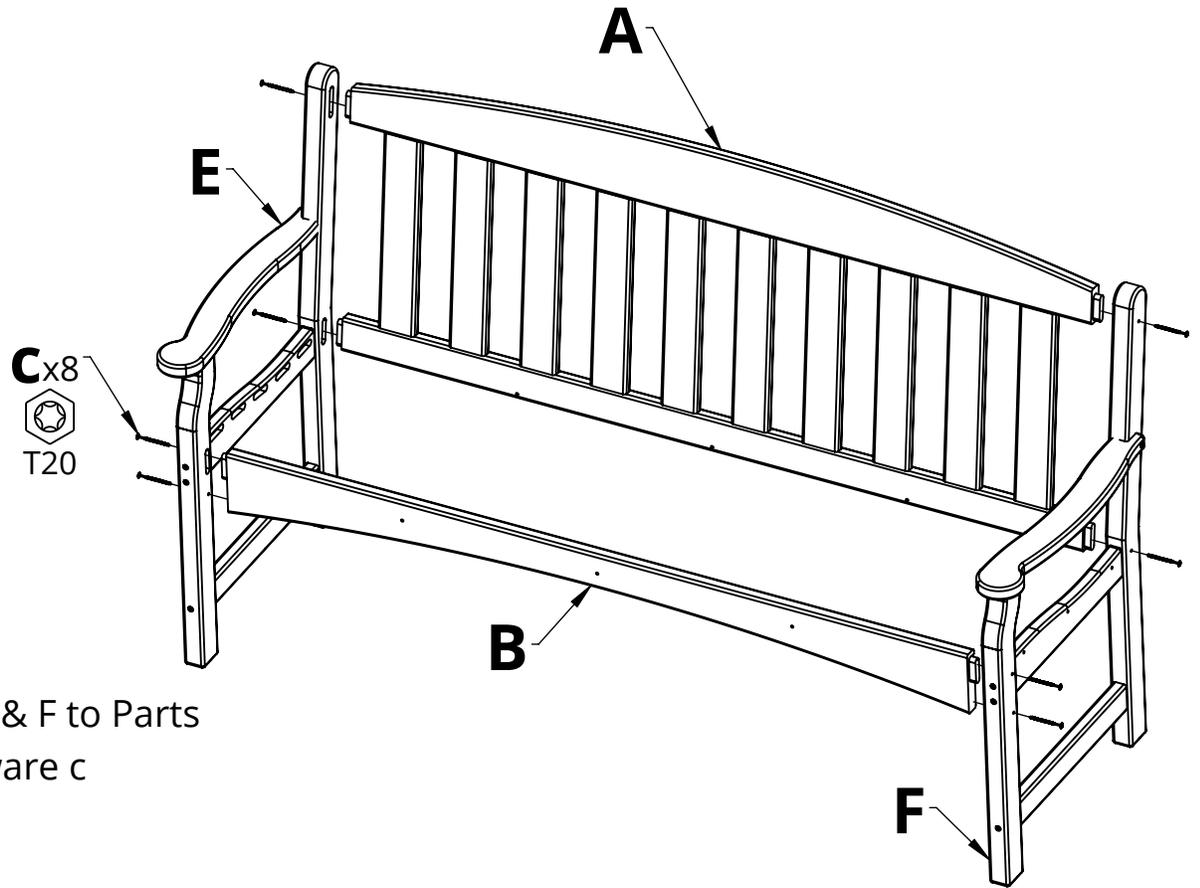
1. Attach Parts E & F to Parts A & B using Hardware c
