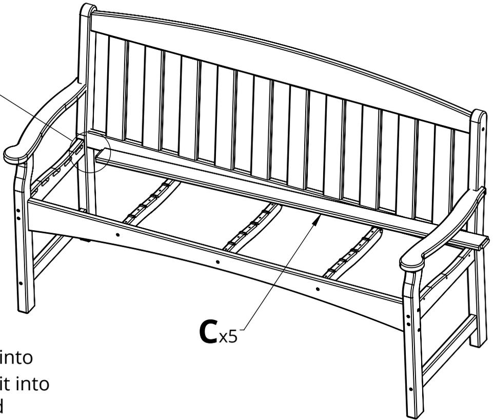
**3.** Slide one end of Parts C into the mortise as shown & flex it into the mortise on the other end
