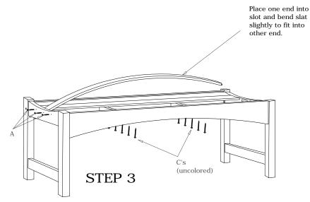
Fit seat slats into bench as shown. From the bottom side use uncolored screws (C) to secure slats. Use screws (A) to attach Side Assemblies to Slats.
