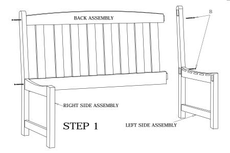
Attach Side Assemblies to Back Assemblies using screws (B) as shown.
